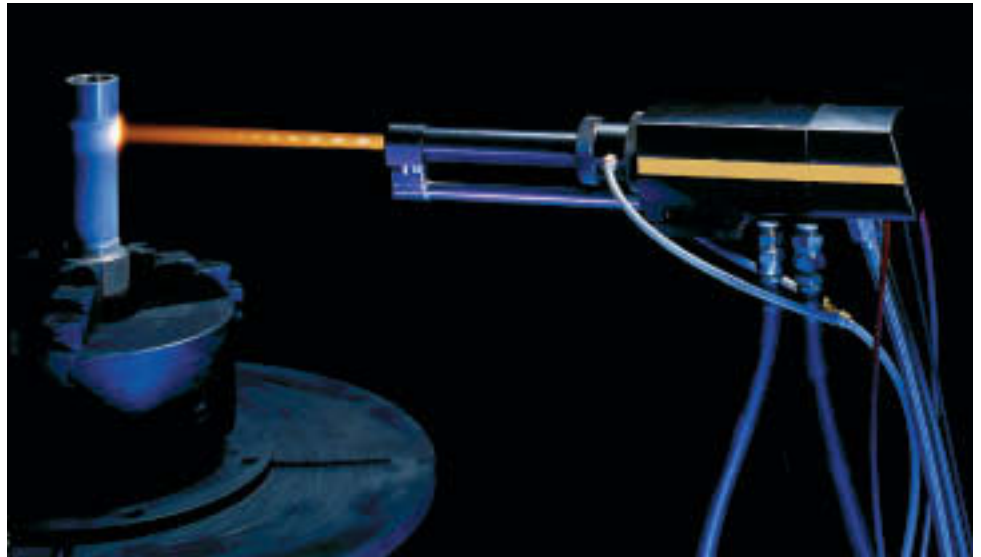
High-velocity oxygen fuel (HVOF) spray can lead to better coatings compared to standard thermal spray in atmospheric conditions.
