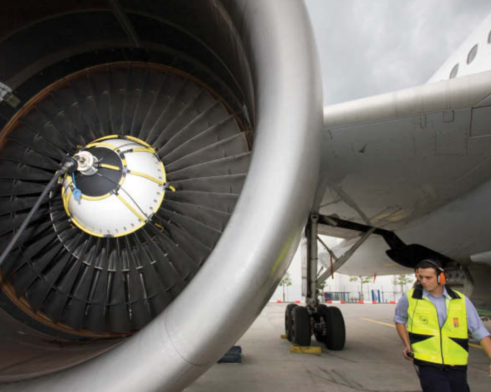
Cyclean engine wash reduces the inner friction of an engine — lowering fuel burn as well as carbon dioxide emissions.
