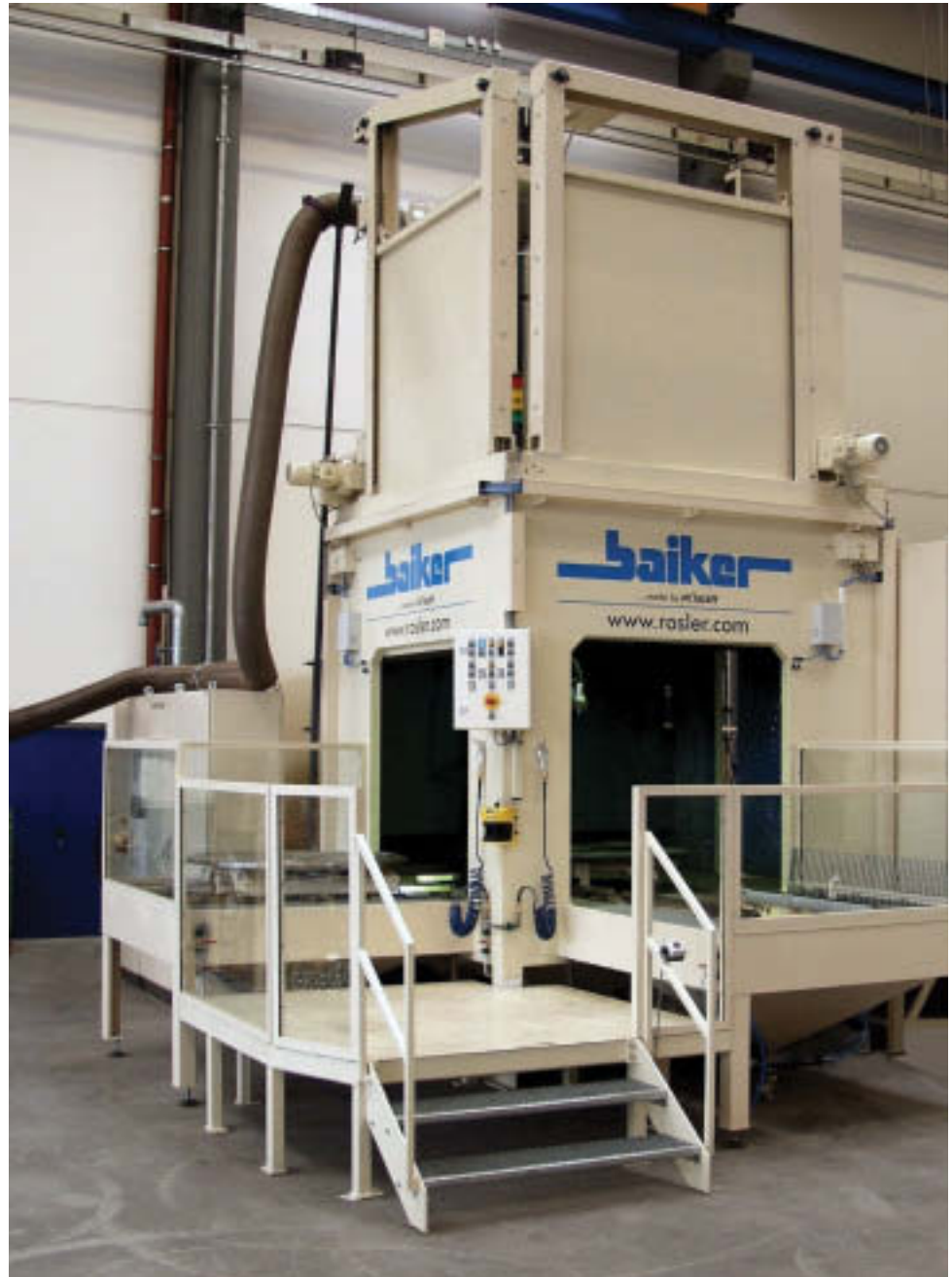
This shot peening system with two load/unload stations is equipped with two independent blast systems and two four-axis gantries guiding the blast guns. This allows the simultaneous peening of the inside and outside surface of the parts.
