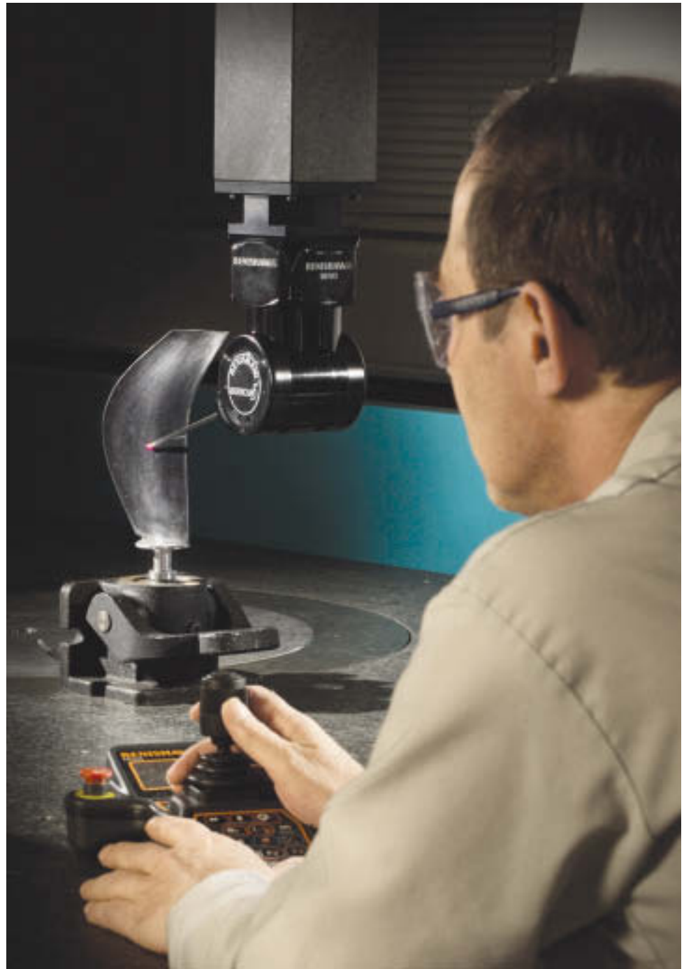
CMM (Coordinates Measuring Machine) inspection of an open rotor reduced-scale blade.
