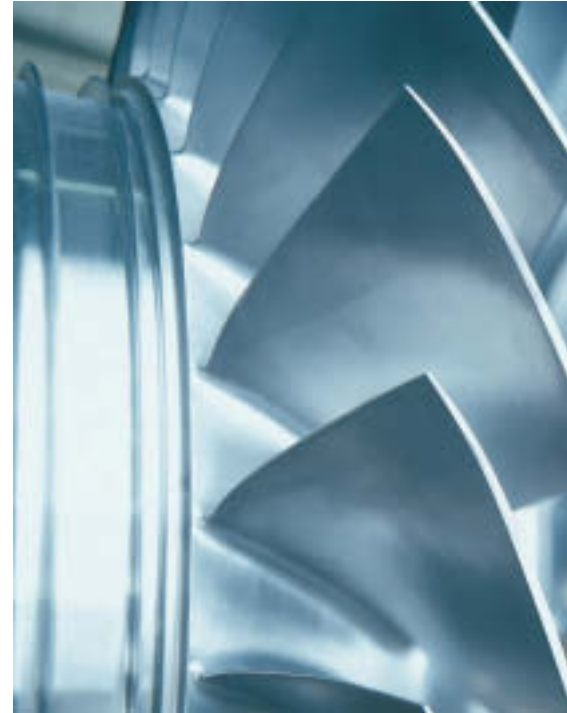
Above - left: At the Munich MTU facility, high-speed milling is used to produce blisks for the EJ200 high-pressure compressor.
