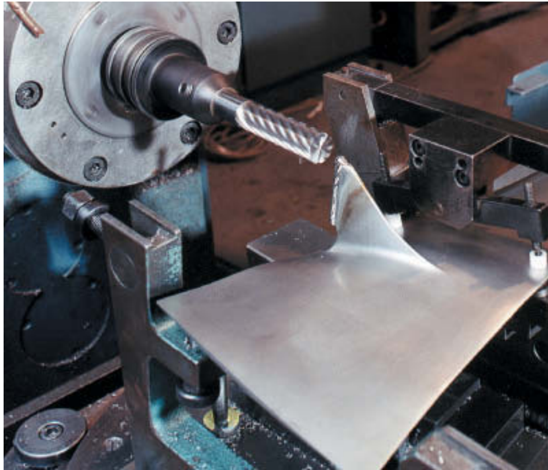
Midspan shrouds are prone to wear and tear, and periodically require material building and machining.
