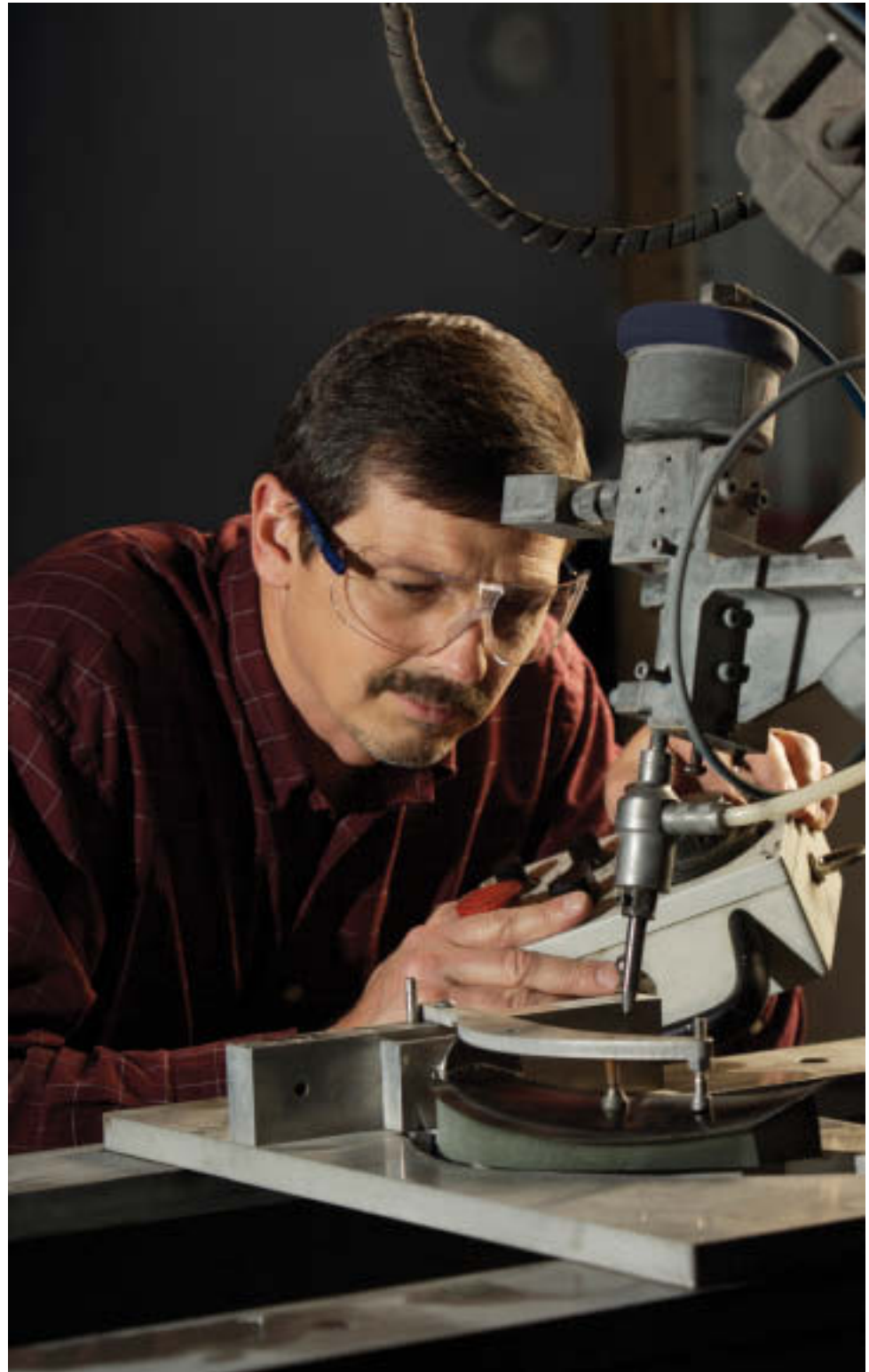
Preparation for water-jet machining of an open rotor reduced-scale blade.
