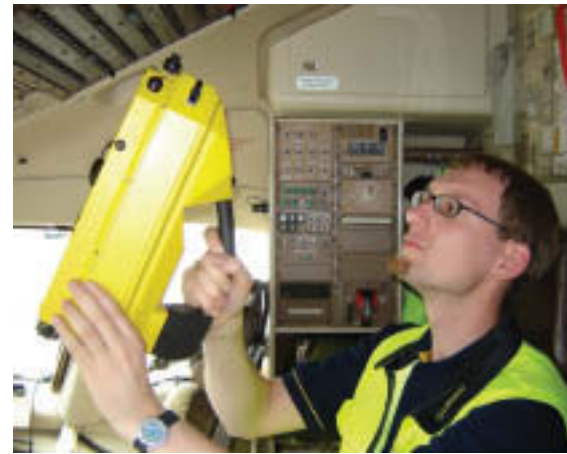
Lufthansa Technik's AeroTracer acts as an "artificial nose" that is capable of detecting and identifying different traces or pollutants in cabin air.
