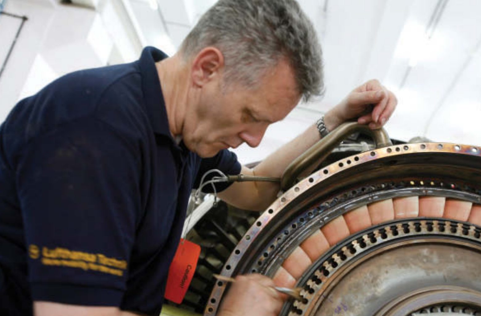
Airline Support Teams can replace a full set or single blades of the CFM56-5 or -7B engines directly at the customer's site.
