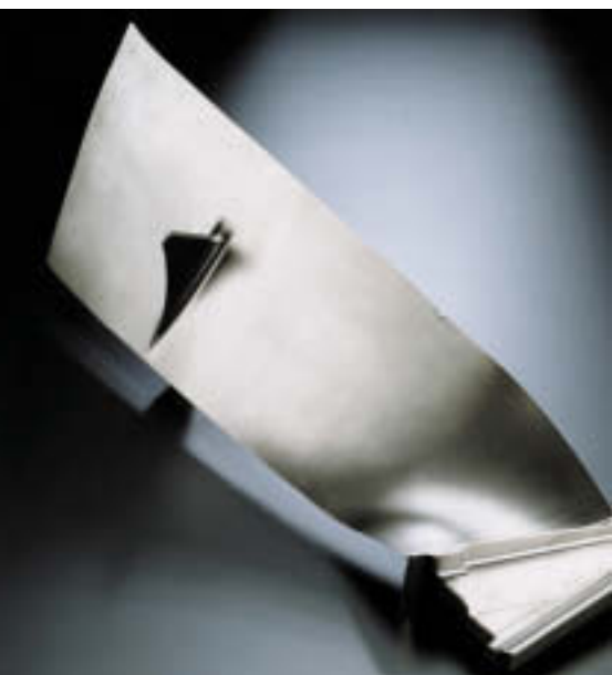
Turbine blades undergo a shot peening process to induce a compressive residual stress in the upper surface layers of the parts. This applies to newly manufactured turbine blades as well as blades that need to be refurbished.
