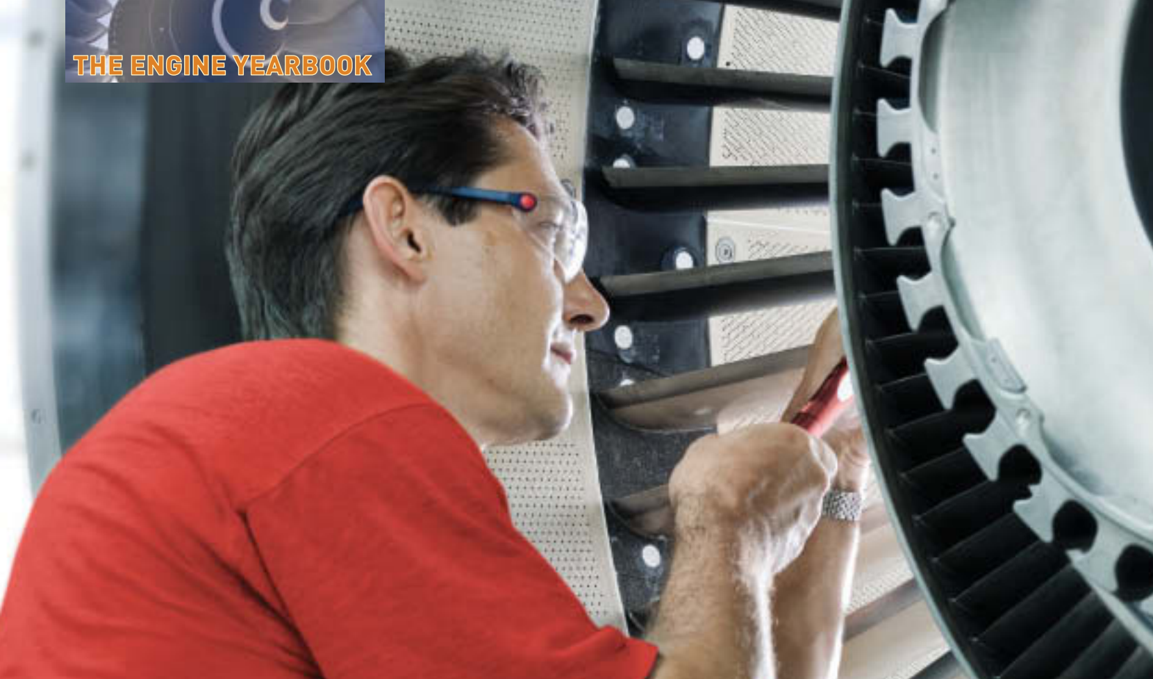
An engineer inspects a fan module.
