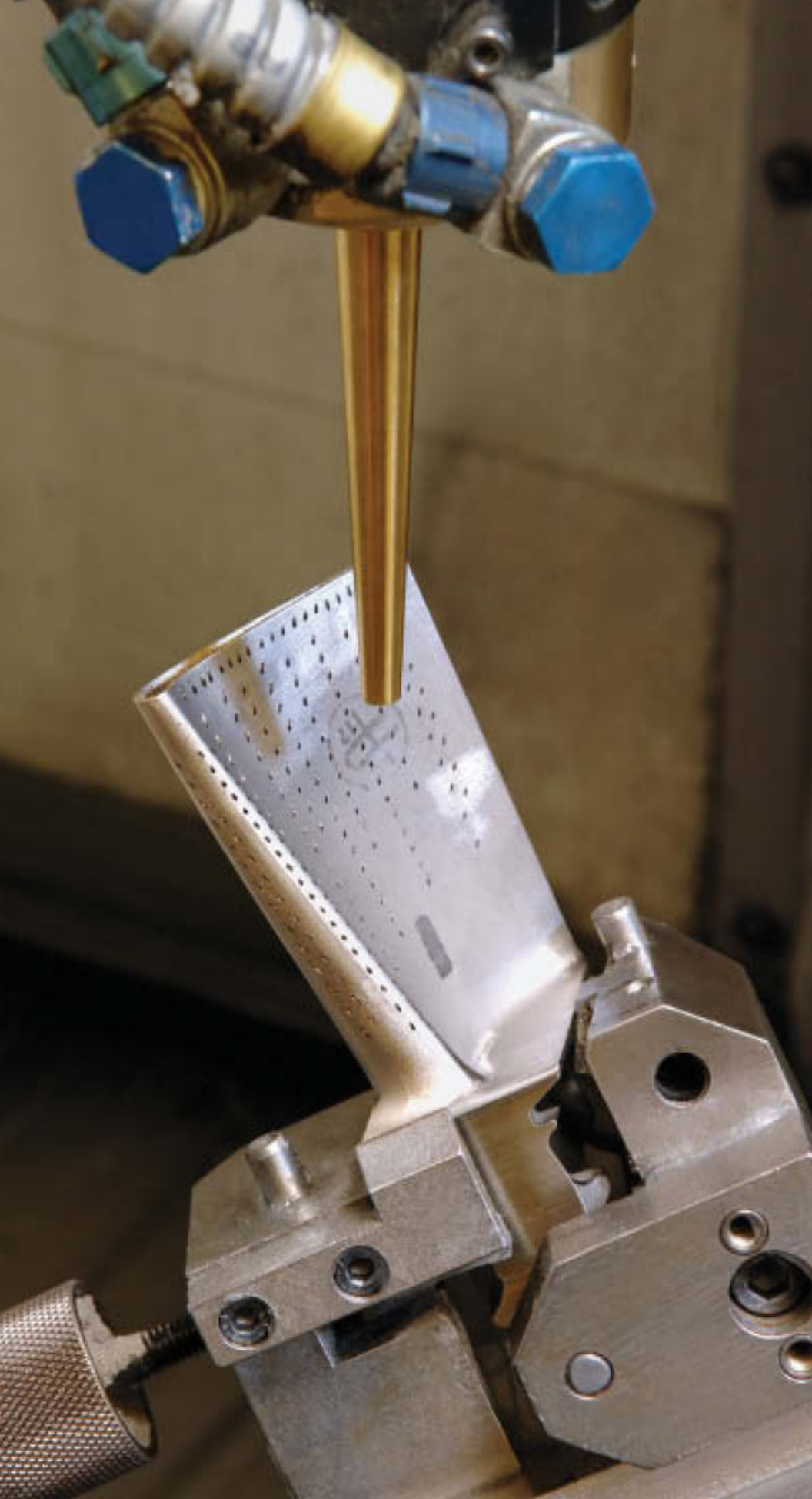
In six minutes the laser drill shoots as many as 180 cooling air holes into a component.
